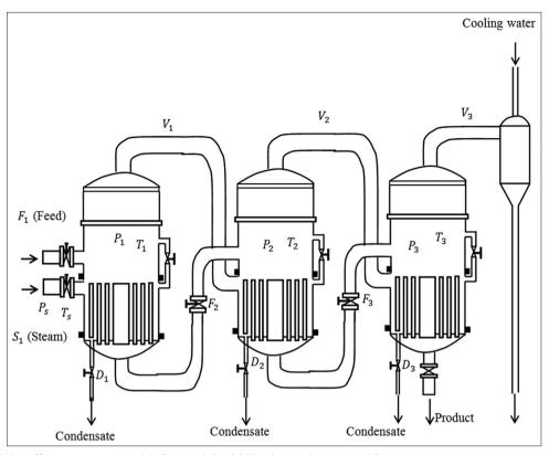
Figure 1a: Multiple effect evaporator with forward feed [Singiresu, S.R. (1996)]
