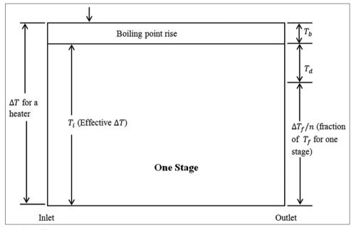
Figure 1c: Boiling Point effect
