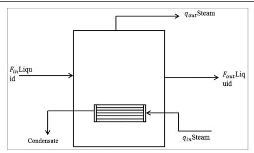
Figure 1b: Individual effect evaporator with forward feed
